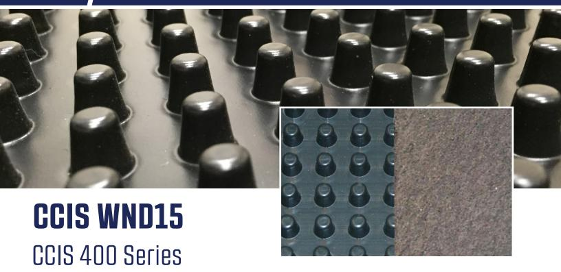
CCIS 400 Series performs a multi-faceted role by providing protection for waterproofing systems and managing subsurface water around building foundations. Soil back fill is retained by a filter fabric while allowing water to pass into the drainage core providing hydrostatic relief. Collected water is then conveyed to a proper collection system.
